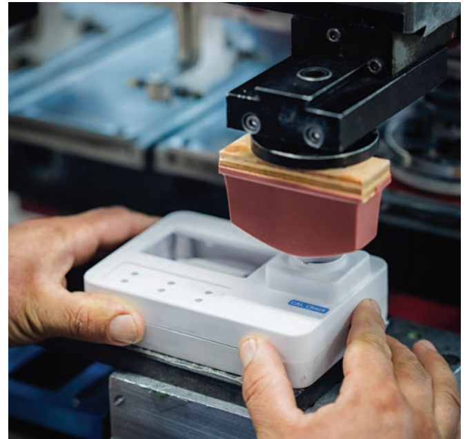
Pad-printing production at Hanna Instruments Nusfalau Science Park
